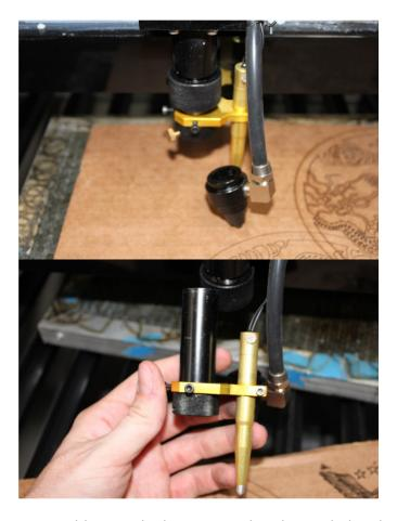
At this point the lens is accessible. Use the lens removal tool provided in the accessory kit to remove the silver screw that is holding the lens in place. There will be a washer that need be removed as well.
