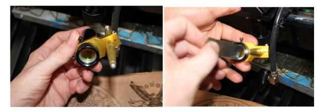
Once the silver screw is removed along with the washer the lens can be switched out. Take note on how the original lens is sitting in the lens holder as that is how the new lens need be installed. Once the desired lens is installed into the lens holder put the laser head assembly
