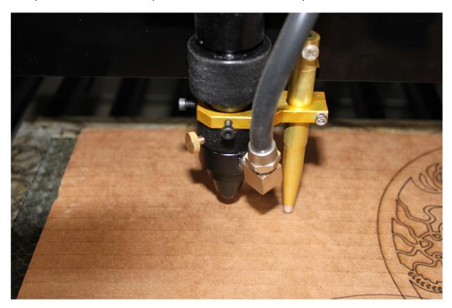
Remove the air assist cone on the bottom of the assembly by unscrewing the gold screw. Once the air assist cone is removed proceed to remove the lens holder from the assembly by loosening the lens holder tensioner.
