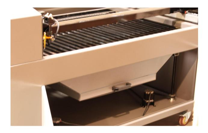
You then need a flat piece of material that you can lay on the knife table. Put the material under the laser head in the bottom left hand corner and raise the z table up until it just touches the auto focus plunger. You will then move the laser head to the upper left corner and check to see if the plunger is the same distance away from the material. Do this to all four corners to ensure that the z table is level.
