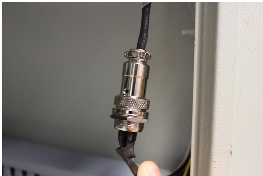
Figure 18 - Rotary Attachment Loose Electrical Connection Detail
