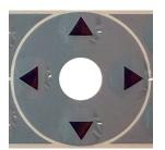
Move the laser head left or right (X axis), forward or rearward (Y axis). Note you can also do this on the Move tab in LightBurn, which also allows you to set a specific distance to move.
